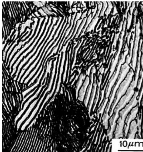
Figure 11-1: The structure of the steel's eutectoid is lamellar (like eutectic phases). We call this phase pearlite. This phase appears in an optical microscope as a dark color and pearl reflections (optical diffraction) from which its name derives.
